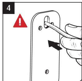
Feed stripped end of cable into the vehicle through 8mm holes. Ensure correct cable goes into correct hole and there is not a crossover. Peel away the other side of the foam like pad.
