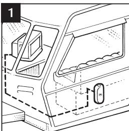
Locate the socket on the vehicle, free of internal features such as cable, seals and any structural components taking into account positions of doors, windows, water, sewerage apertures. You may wish the cable to enter the vehicle under the seat, in a cupboard or somewhere out of sight. Ensure you have easy access from the inside to feed the cable through. Take care not to trap cable.
