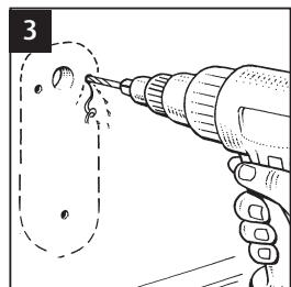
Drill holes with the specified drill bits below. Treat/seal any exposed materials as required to prevent decay. Once these are drilled out, peel off one side of the adhesive backing on the foam like pad. Stick this to the vehicle making sure all the holes are aligned precisely.
