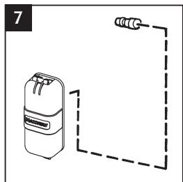
Route cable inside the vehicle to your TV or receiver. For the best interference free reception do not run parallel to electrical or other power cables. Take care not to trap cable. Fit 'Coax' Plug. See page 4 for fitting details.
