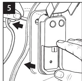
Carefully offer up socket to vehicle, correct alignment of holes is critical, someone may need to be inside the vehicle pulling through any cable slack.
