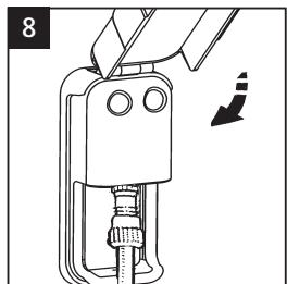
Route cable outside the vehicle from aerial and connect (see above). Close lid, \*lid closes in intermediate position when external cable are connected.
