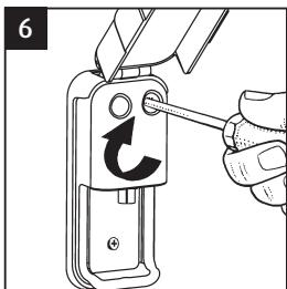
Locate and fit all self tapping screws. Tighten clockwise, being careful not to over tighten.
