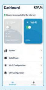
Switch internet source between SIM card (data) and Wi-Fi
