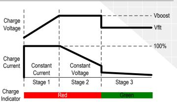
During stage 1 the battery voltage is increased gradually while the current is limited to start the charging process and protect the battery. At stage 2 the voltage rises to 14.4V (Vboost) to deliver the bulk charge to the battery. When the battery is charged, the voltage is decreased at stage 3 to 13.6V (Vflt) to deliver a float charge to maintain the battery in the fully charged state. The charger can be left switched on continuously as required.
