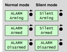
When in basic mode and the alarm is armed the top & bottom buttons will be disabled and the display will show one of the screens shown left.
